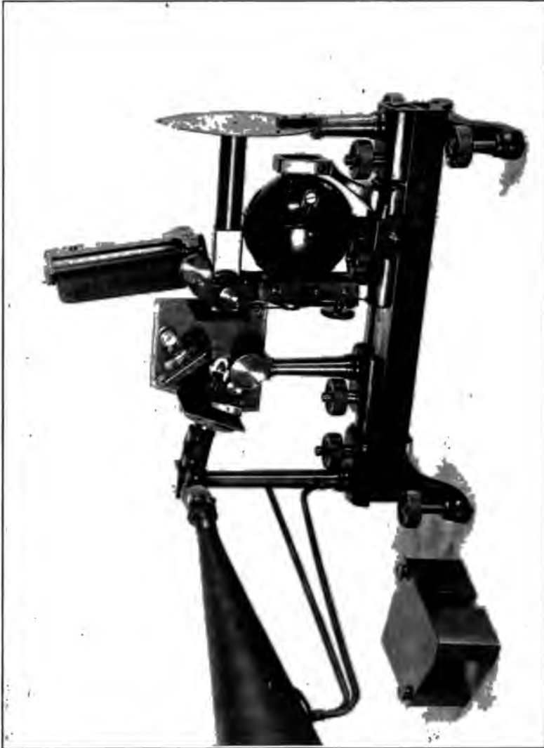
FIG. 69. Projection phonodeik for rendering sound waves visible to a large audience.
